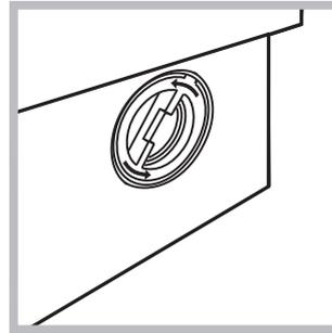
1. unscrew the lid by rotating it anti-clockwise (*see figure*): a little water may trickle out. This is perfectly normal;
